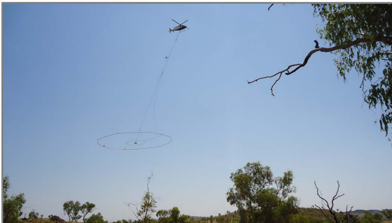
Photo 1: Geotech Airborne Geophysical Surveys flying the VTEM Super Max survey at the McIntosh Flake Graphite Project
